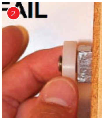
This bolt end is an unsafe protrusion.
