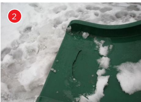
This tear could be an entanglement hazard.
