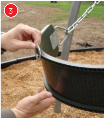
Test swings for protrusion hazards with this special gauge.
