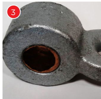
3 This bushing (red) is worn and should be replaced.
