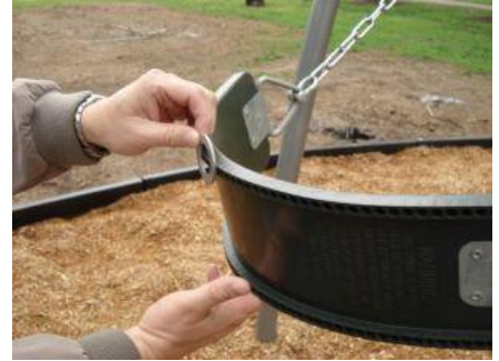
For suspended components use 1 ¼" diameter, 1/8" extension gauge
